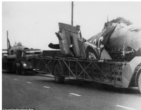
‘Queen Mary’ transporters in action loaded with damaged aircraft
