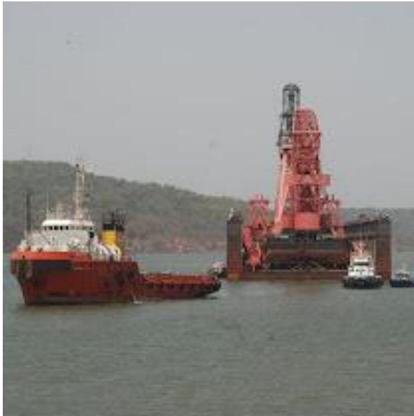
The wet tow in the Vashishti River on passage to the shipyard
