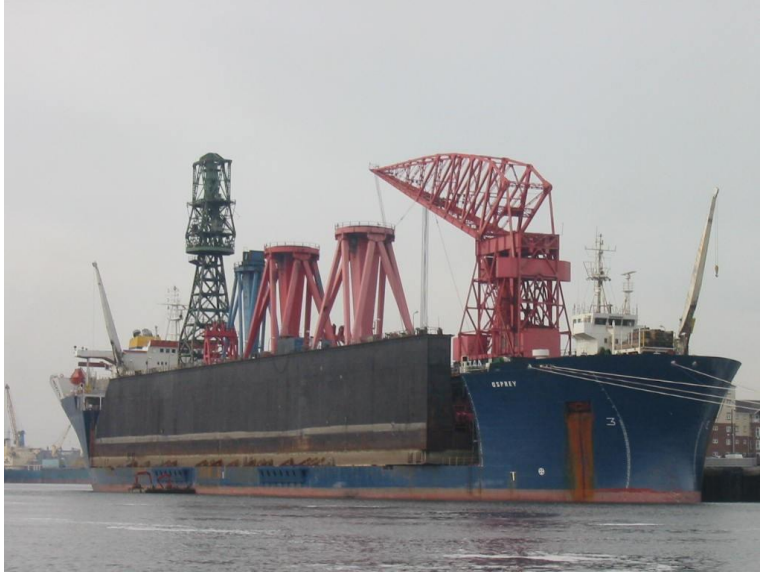
Osprey deballasted, floating dry dock secured on deck
